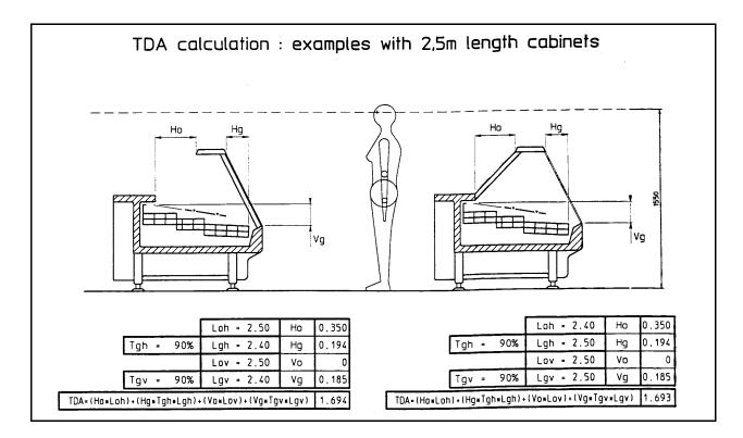
Fig.3. Evaluation of total display area (T.D.A) for a refrigerated service counter.
