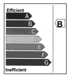
Fig.1.The indication of energy efficiency (here efficiency class B) as it appears on the physical European energy label, with the unmistakable "arrows".
